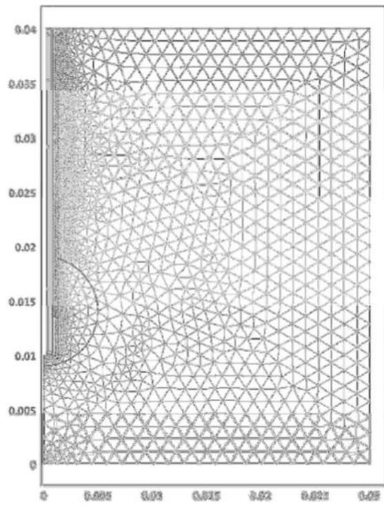
**Figure 3.** Plot of the whole model with mesh grids. This FEM model contains 4835 elements.
