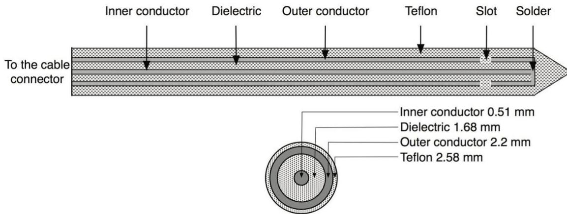
**Figure 1.** Cross section and schematic of the coaxial slot applicator.
