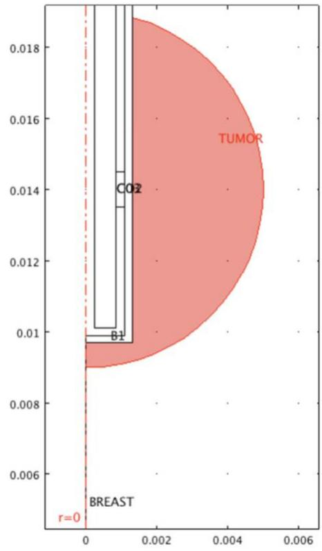
**Figure 2.** Axisymmetric CEM model in the vicinity of the tip of the coaxial slot antenna. The vertical axis corresponds to the longitudinal axis of the antenna while the horizontal axis corresponds to radial direction.
